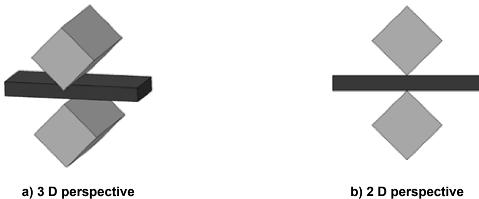
Figure F.1 — Principle of wedge penetration test
